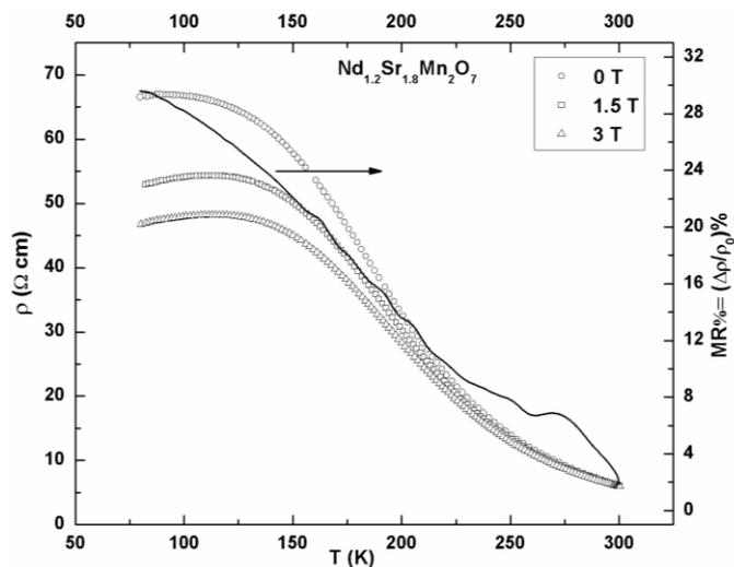
Fig. 1 Variation of electrical resistivity and MR with temperature
