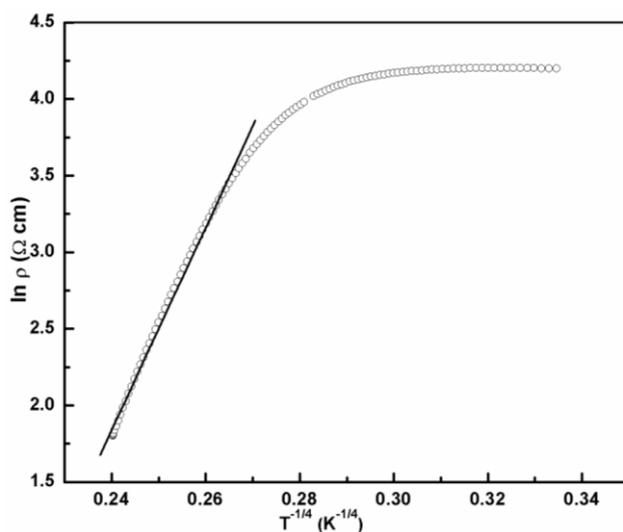
Fig. 2 Plot of  $\ln \rho$  vs.  $T^{-1/4}$  for  $Nd_{1.2}Sr_{1.8}Mn_2O_7$
