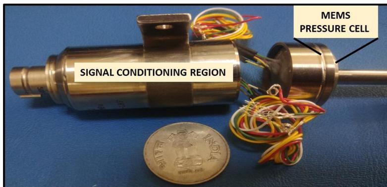
Figure 5.0 Satellite version MEMS pressure transducer cut opened view after radiation test
