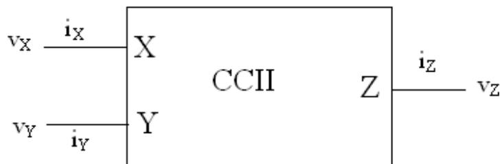
Figure 2. second generation current conveyor
