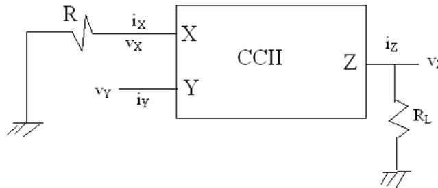
**Figure 3: VCVS using CCII+**
