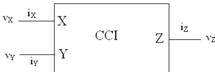
Figure 1: First generation current conveyor
