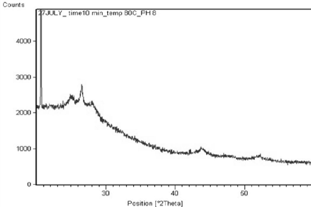
Figure 4:- XRD of CdS thin film
