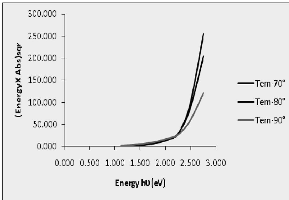
Figure 3:- Band gap variation for CdS thin film at different temperature.
