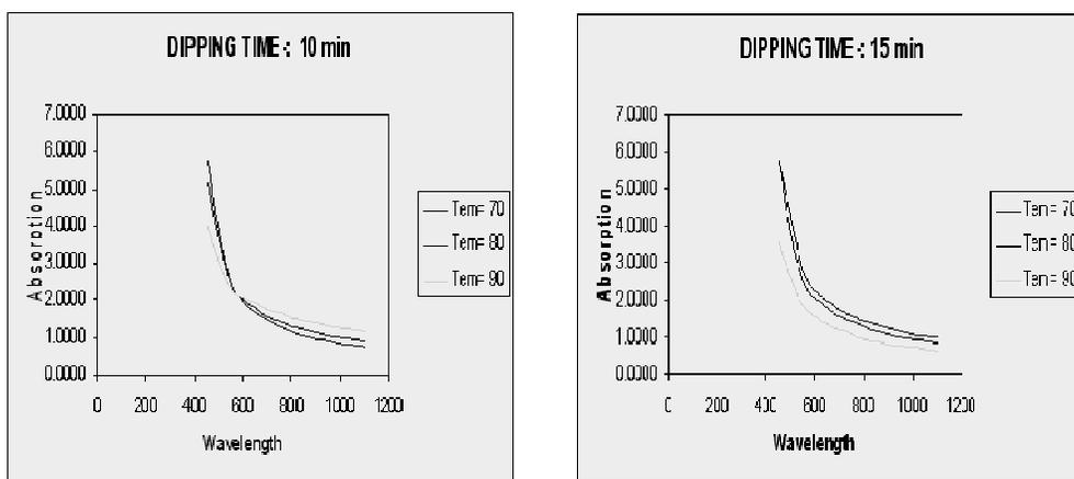
Figure 2(a, b):- Absorption - Wavelength graph for CdS thin film at diff. dipping time.
