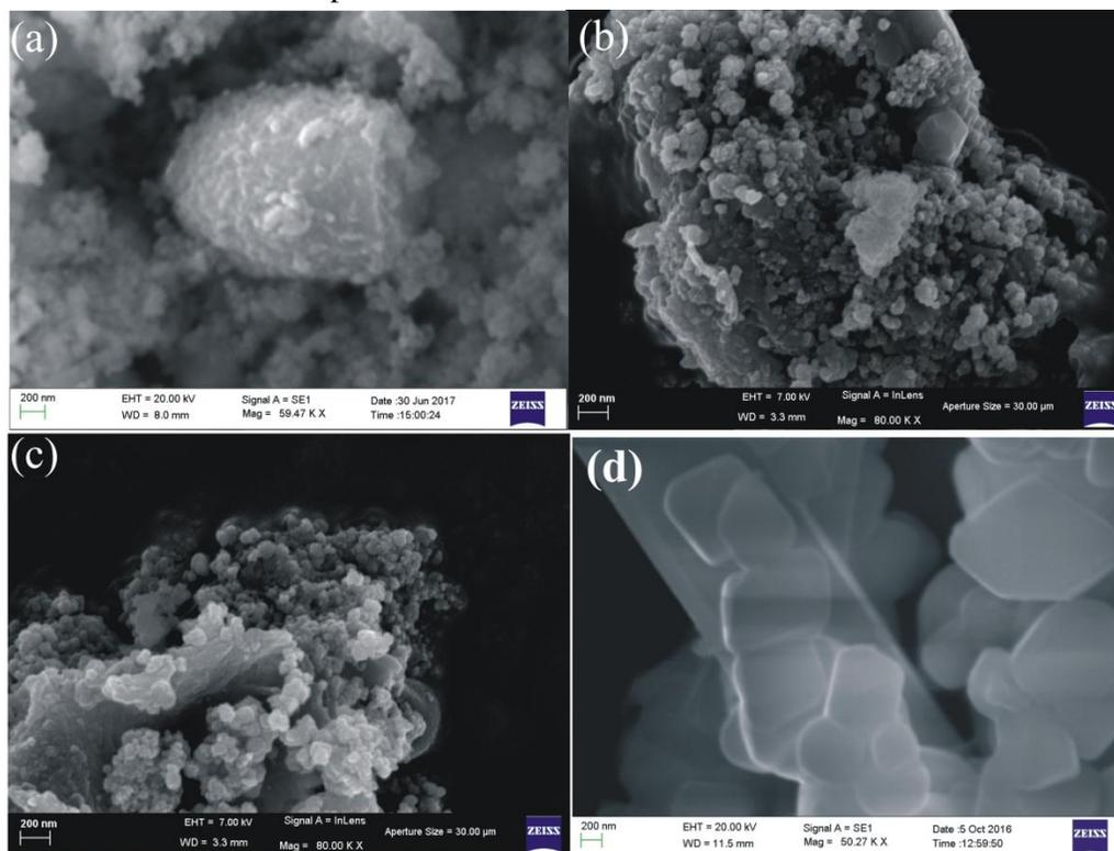
**Figure 3.** SEM image of  $Mn_2O_3$  at 200 nm magnification 59.99 K X with CTAB variation (a) 0 mg, (b) 20 mg, (c) 50 mg and (d) 100 mg.
