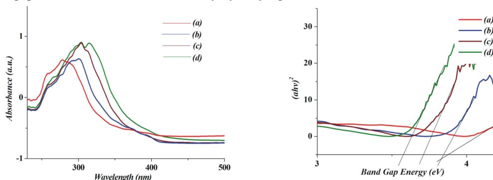
Figure 4. UV-visible spectra of  $Mn_2O_3$  with the variation of amount of CTAB (a) 0 mg, (b) 20 mg, (c) 50 mg and (d) 100 mg (inset) Tauc plot indicating band gap.
