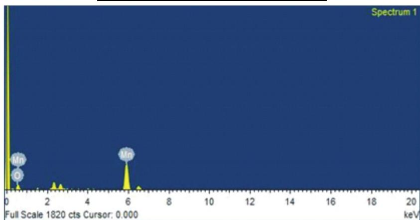
**Figure 2.** EDS spectra of  $Mn_2O_3$  without CTAB indicating elemental composition.
