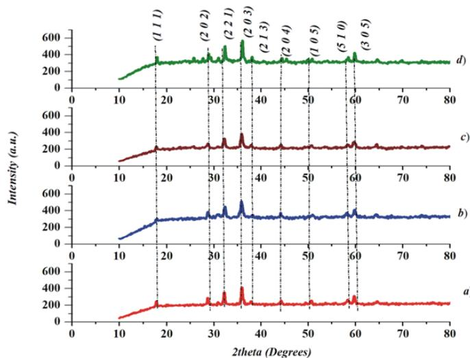
**Figure1.** XRD of synthesized  $Mn_2O_3$  with the variation of the concentration of CTAB (a) 0 mg, (b) 20 mg, (c) 50 mg and (d) 100 mg.
