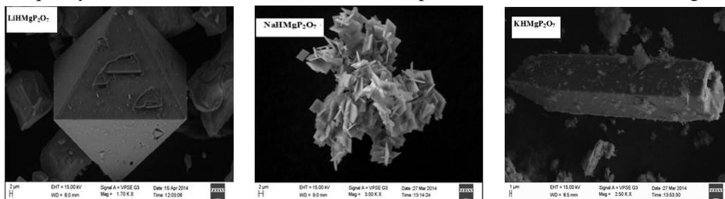
**Fig.1: SEM photograph of  $M^+-HMg-P_2O_7$  ( $M^+=Li, Na$  and  $K$ ) materials**
