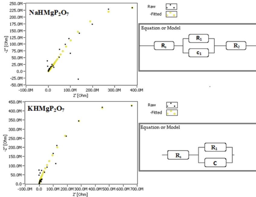
**Fig.4: cole- cole plot and equivalent circuit**
